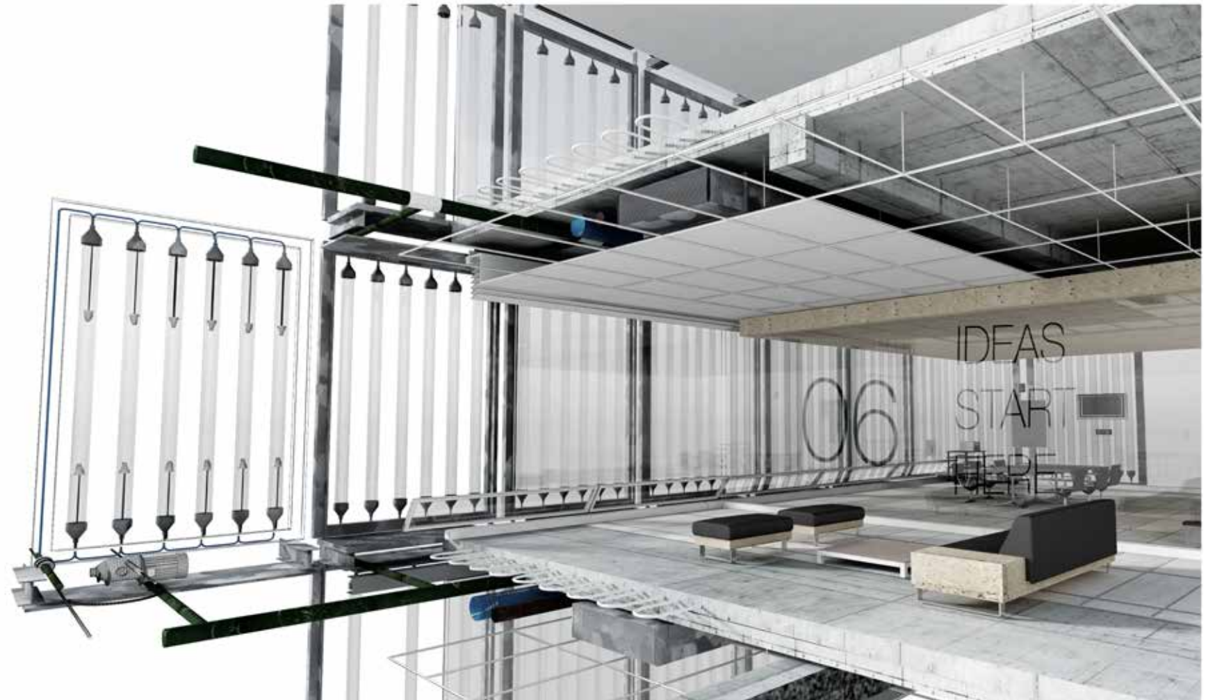
Fig 05: External tube facade detail: bio-adaptive facade of microalgae
